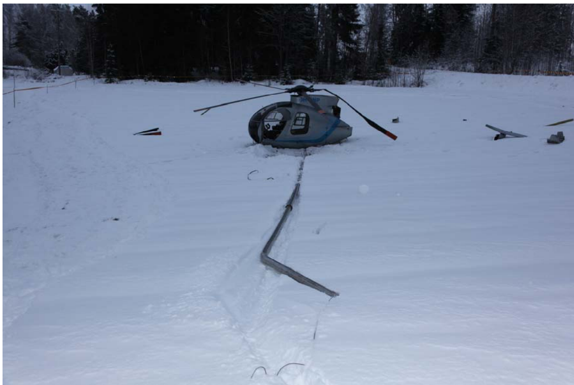
Figure 3. The broken saw suspension bar, photographed from the direction where the helicopter came from.
