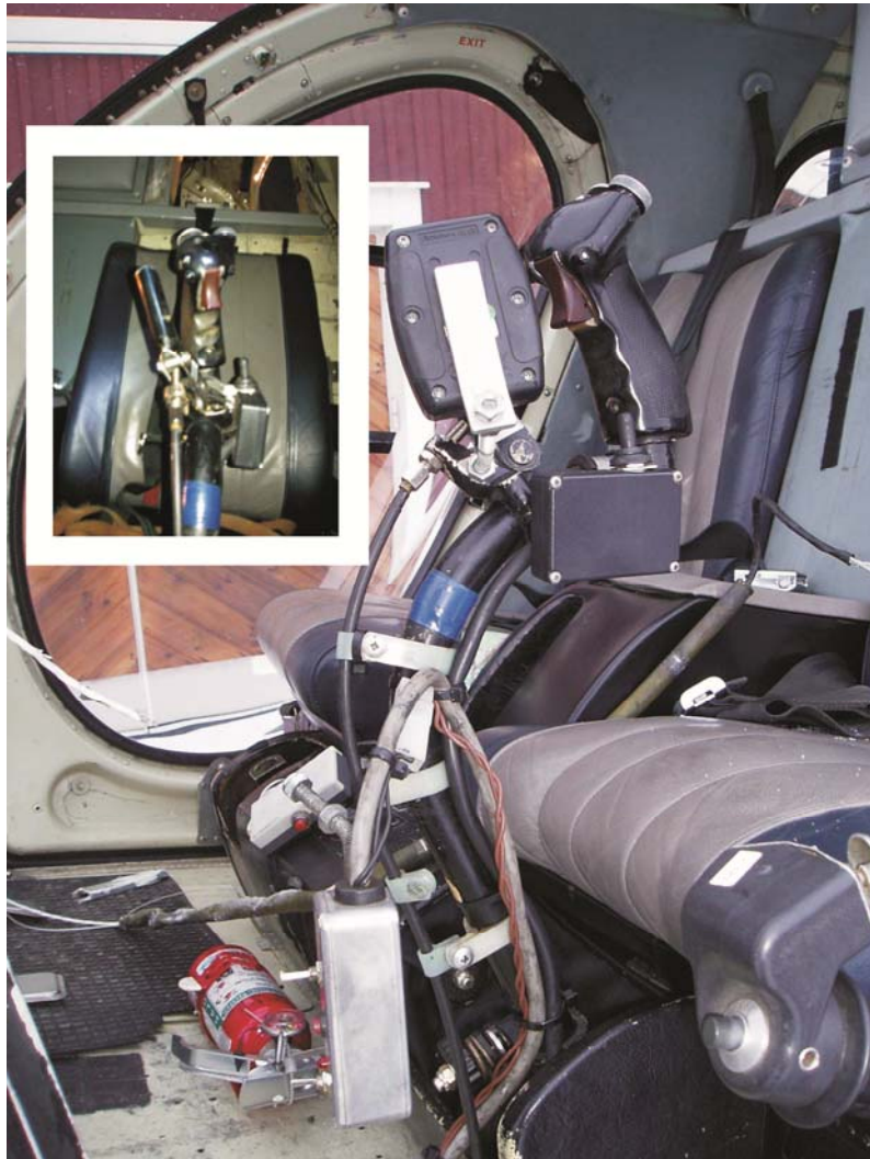
Figure 6. The layout of the sawing unit's controls and the external cargo emergency release handle, photographed from the side and the front.
