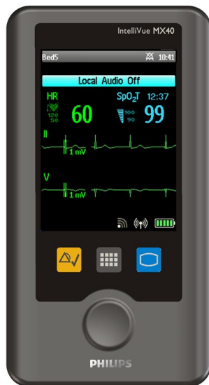
Figure 3. The touch screen on the Philips IntelliVue MX40 device displays measurement numerics, information fields, alarm fields, waveforms, SmartKeys and menus. (Picture: Philips) 15
