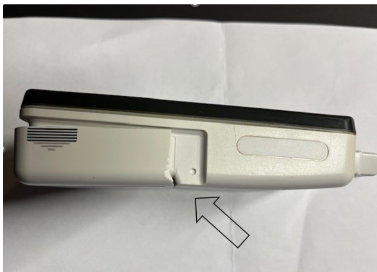
Figure 6. Broken hinges on the battery compartment door and a broken clip in the compartment. (Photo: SIAF)
