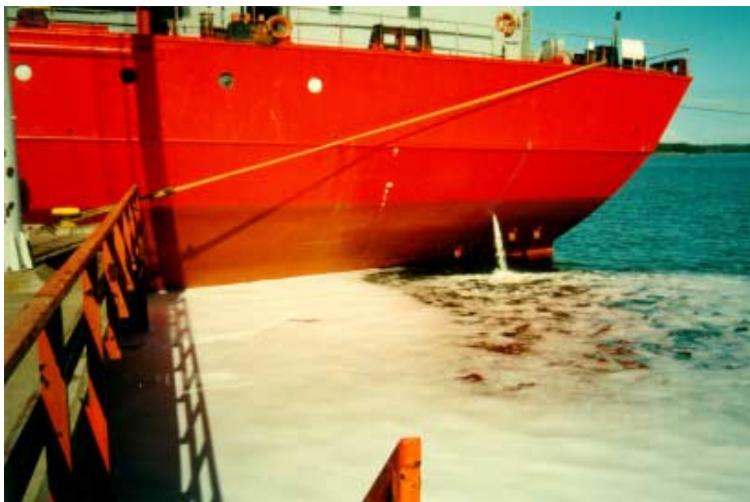
Figure 8 Foam in the sea after the leak. The substance coming out of the hole at the stern is cooling water for auxiliary machine and not related to the accident.
