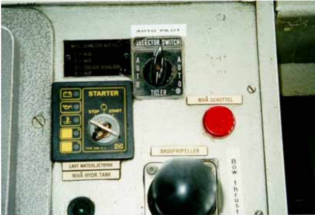
Figure 14. Selector switch for autopilot and manual steering.
