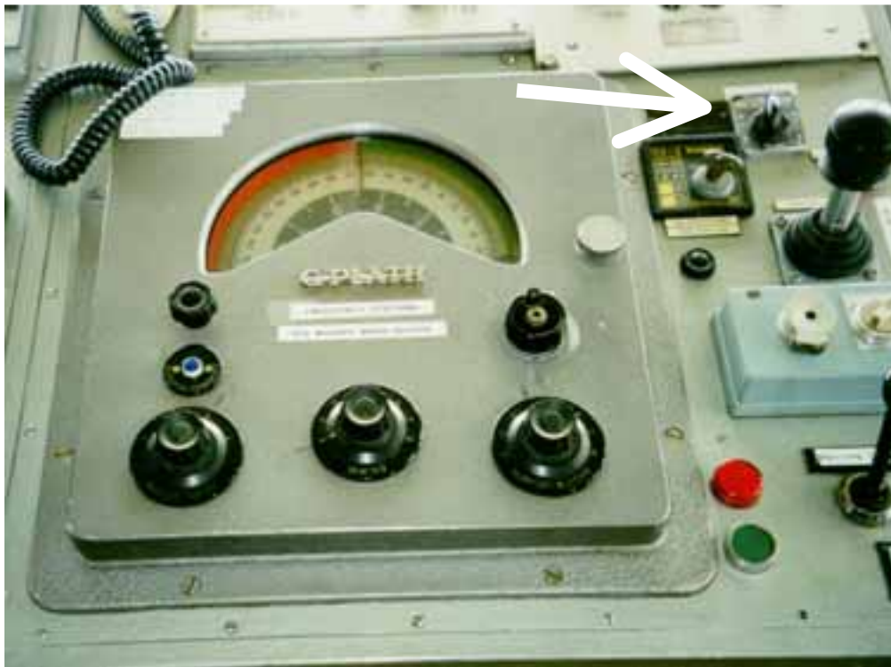
Figure 12. Photograph of the autopilot with the switch for the autopilot and manual steering (marked with arrow).
