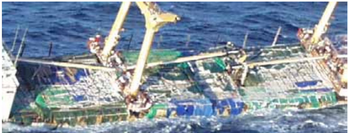
Figure 14. Shifted deck cargo, close-up of figure 2
