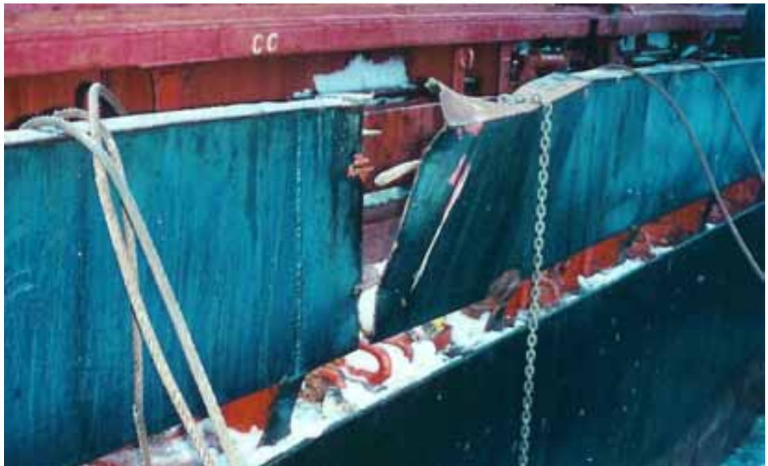
Figure 18. Damage to the railing
