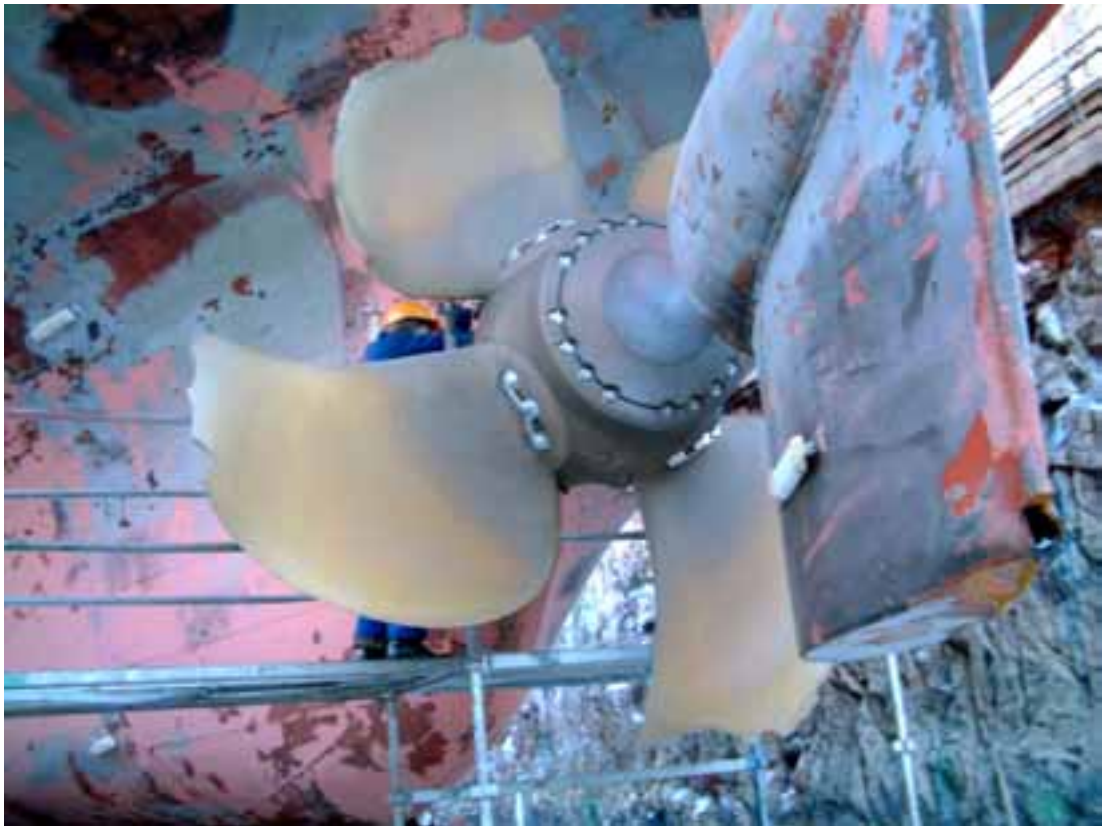
Figure 10. Damage to the propeller, all blades damaged
