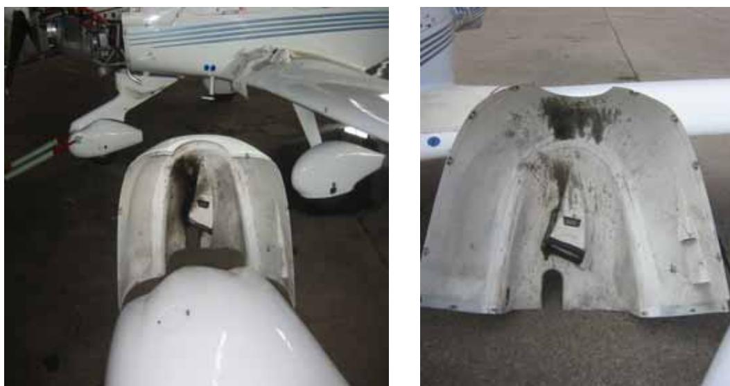
Figure 8. Oil leak traces on the lower engine cowling. Left photo taken on 17 April 2007. Right photo taken on 26 April 2007.
