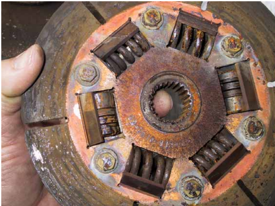
Figure 2. The badly damaged clutch plate
