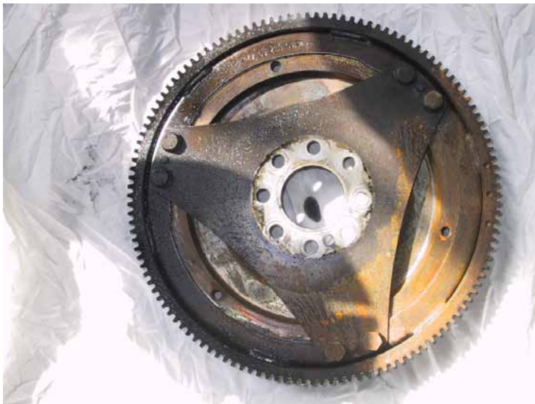
Figure 3. The oily rear surface of the flywheel
