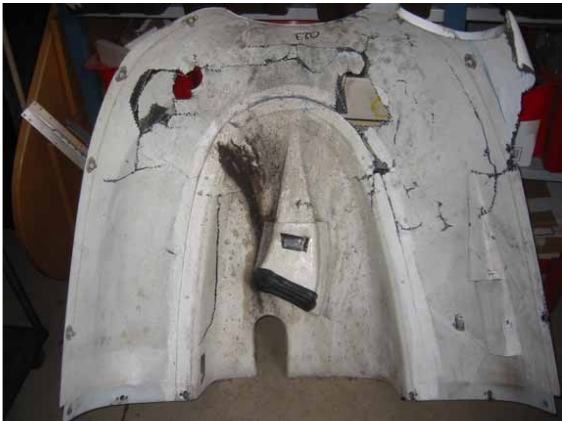
Figure 9. Oil leak traces after the emergency landing
