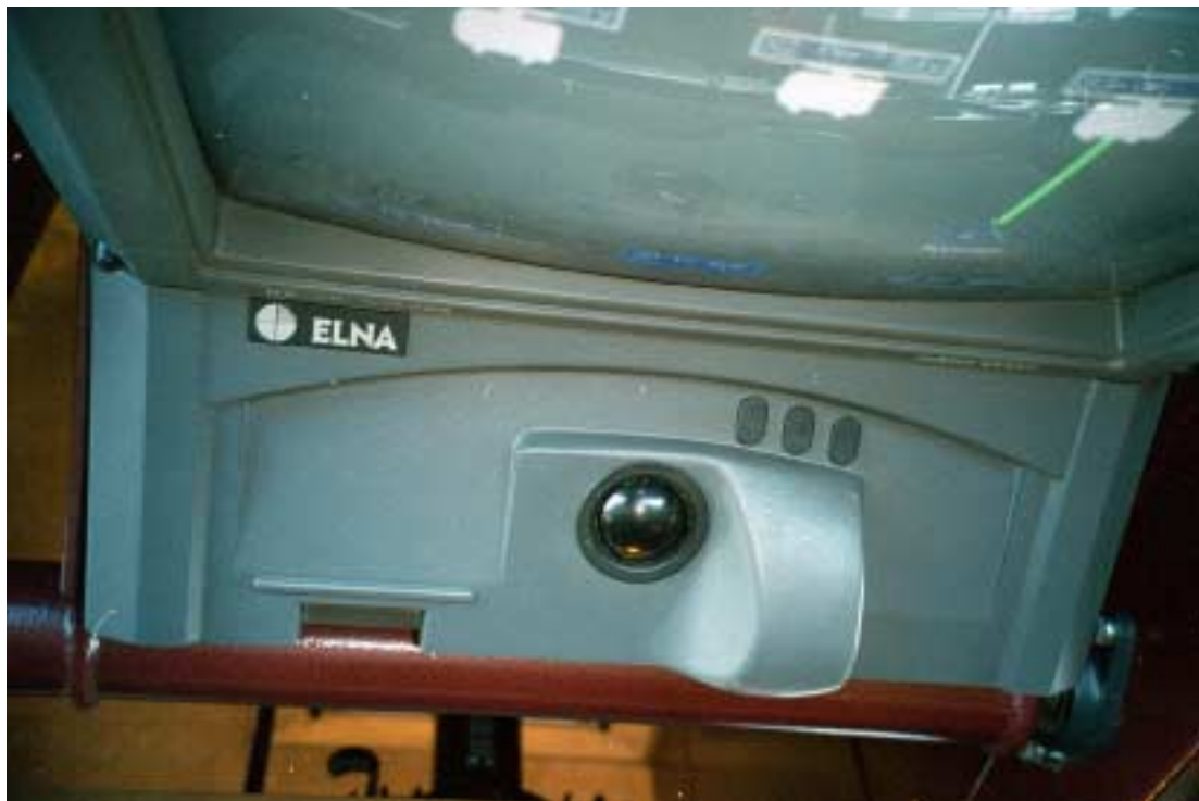
Figure 9. Keyboard of Kelvin & Hughes radar.
