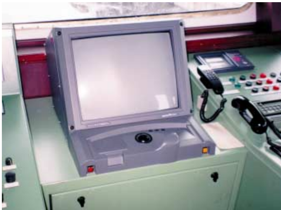
Figure 6. Kelvin & Hughes marine radar
