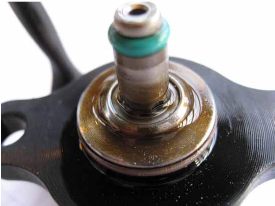
Figure 5 Metal particles in the pressure control valve
