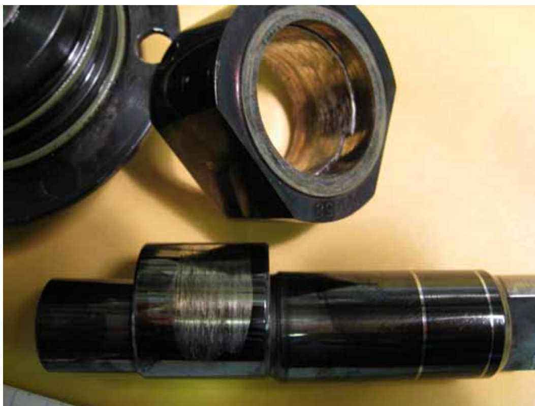
Figure 4 Damages of the eccentric cam and the driveshaft on the HP pump.
