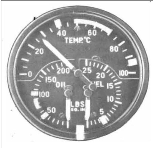
Figure 5. The gage unit with the fuel pressure gage in the lower right-hand quadrant. The thick white line indicates the normal pressure range. (Photo: SIAF)
