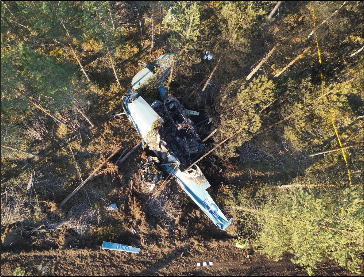
Figure 15. The wing assembly separated, and the fuselage was consumed by fire. (Photo: SIAF)
