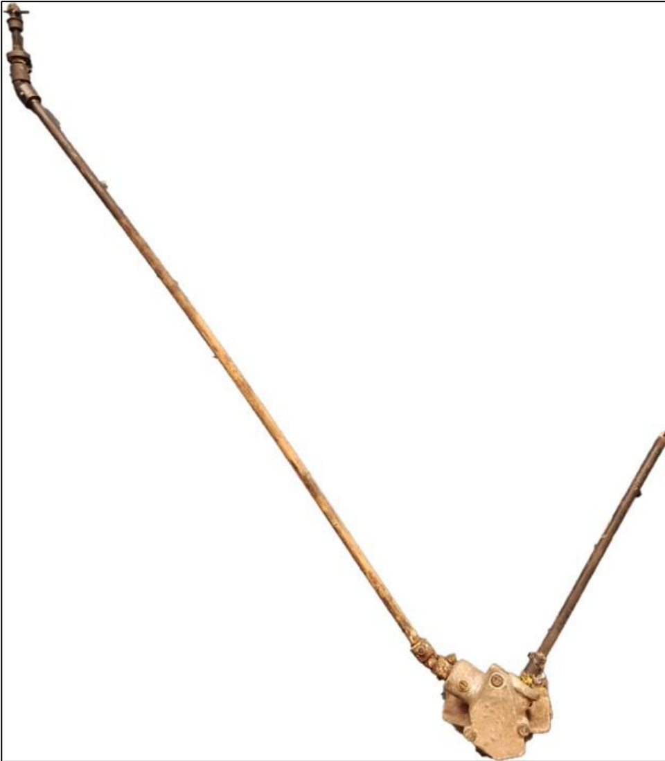
Figure 24. The fuel selector mechanism. The fractured rod that was connected to the rear cockpit selector is on the right, and the rod from the front cockpit selector is on the left. (Photo: SIAF)
