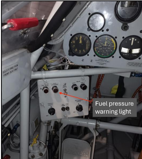
Figure 8. The location of the fuel pressure warning light in the rear cockpit of OH-NAT. (Photo: Airplane owner, edited by SIAF)
