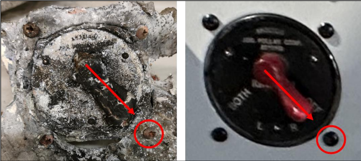
Figure 19. The ignition switch was found in OFF position. The right-hand inset shows the switch in its original condition. (Photos: SIAF, airplane owner, edited by SIAF)
