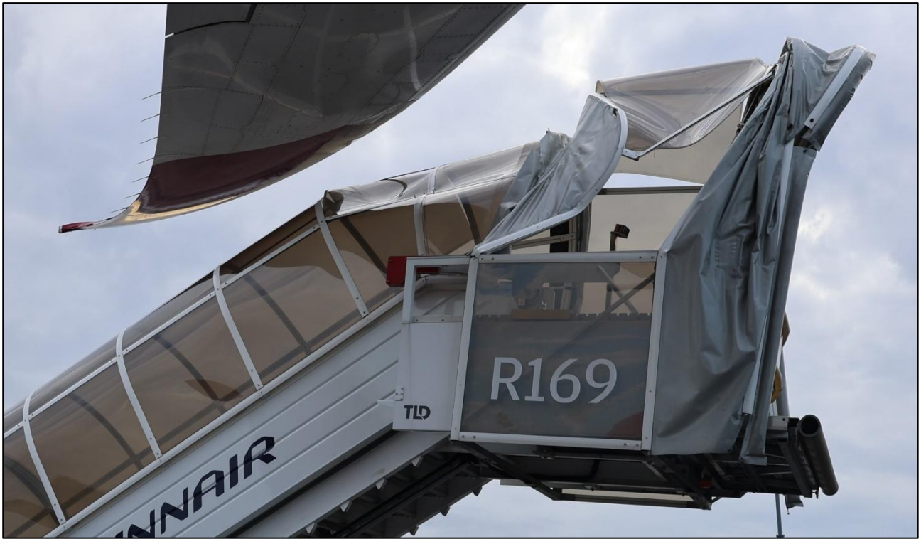
Figure 3. Damaged stairway canopy. (Photo: SIAF)
