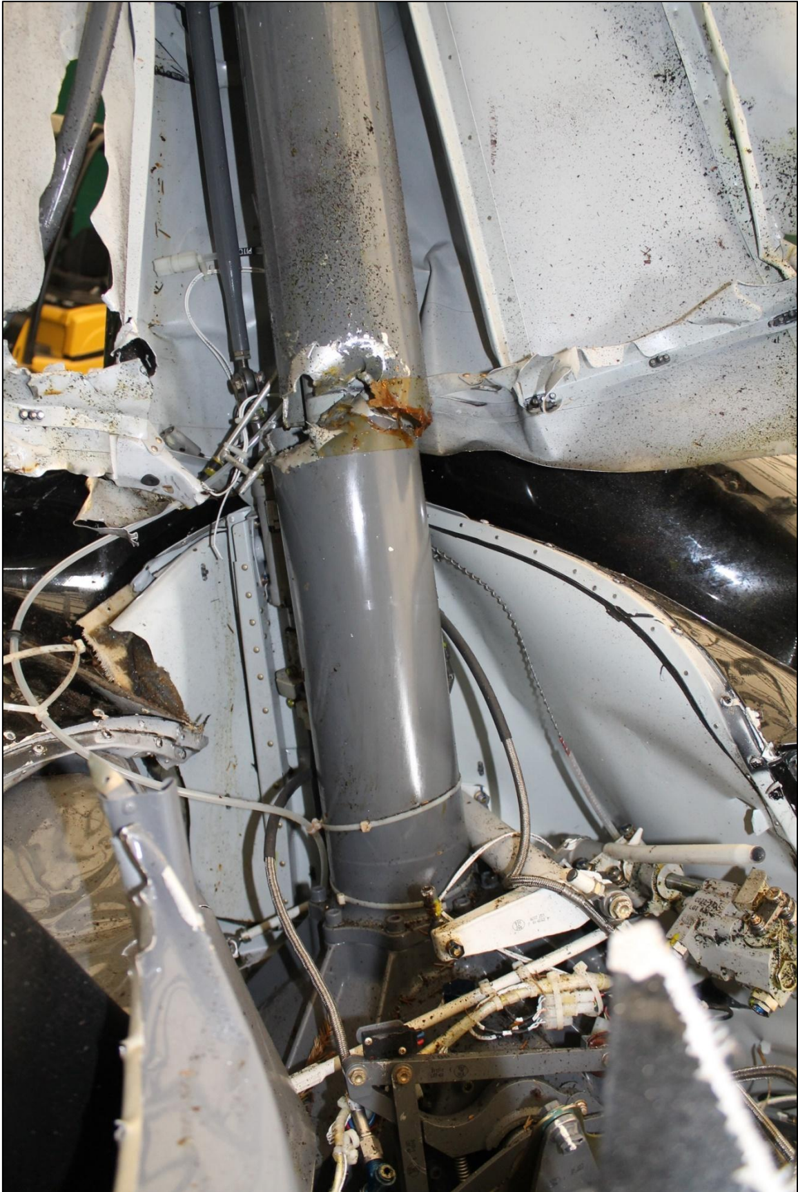
Figure 11. The main rotor mast of OE-XOS was fractured about 40 cm above the main gearbox. (Photo: SIAF)
