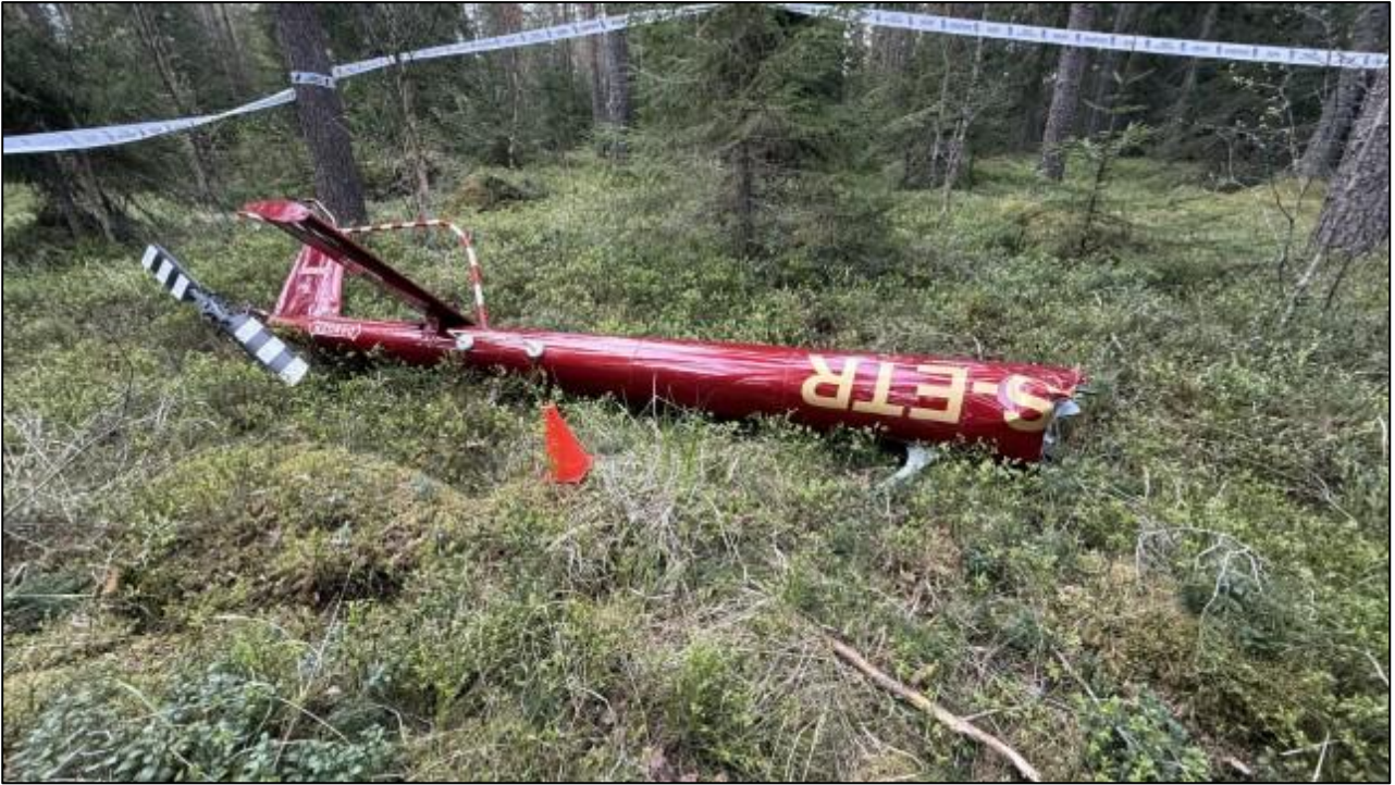
Figure 8. The tailboom of ES-ETR separated during the collision sequence. (Photo: SIAF)
