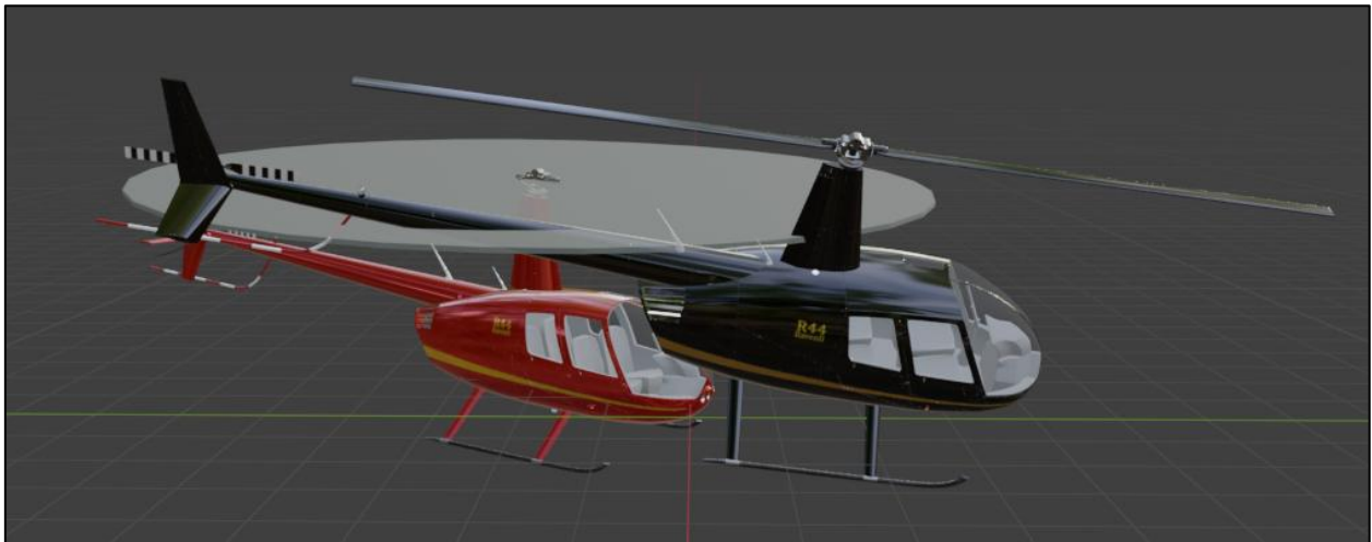
Figure 14. Estimated attitude of the helicopters on impact, based on damage described in this paragraph. (Figure: SIAF)
