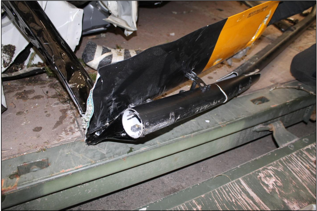
Figure 13. The rear section of the right skid and strut of OE-XOS and a main rotor blade of ES-ETR. Matching damage is apparent. (Photo: SIAF)
