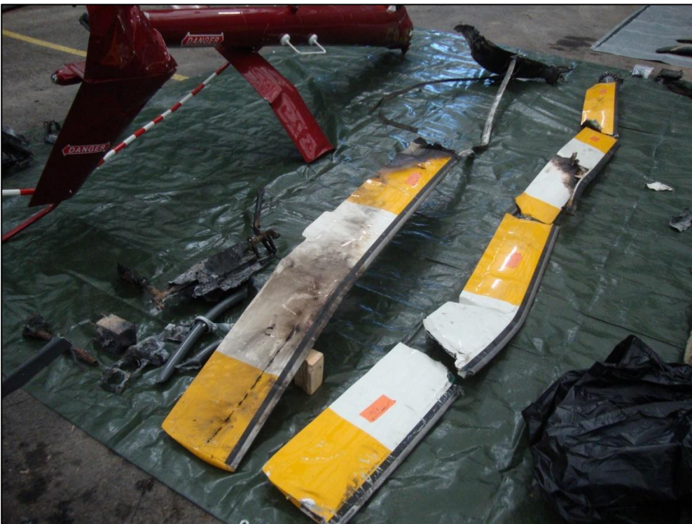
Figure 9. The main rotor blades of ES-ETR. One blade was destroyed between the root and mid-span, while the other broke into four sections. (Photo: SIAF)
