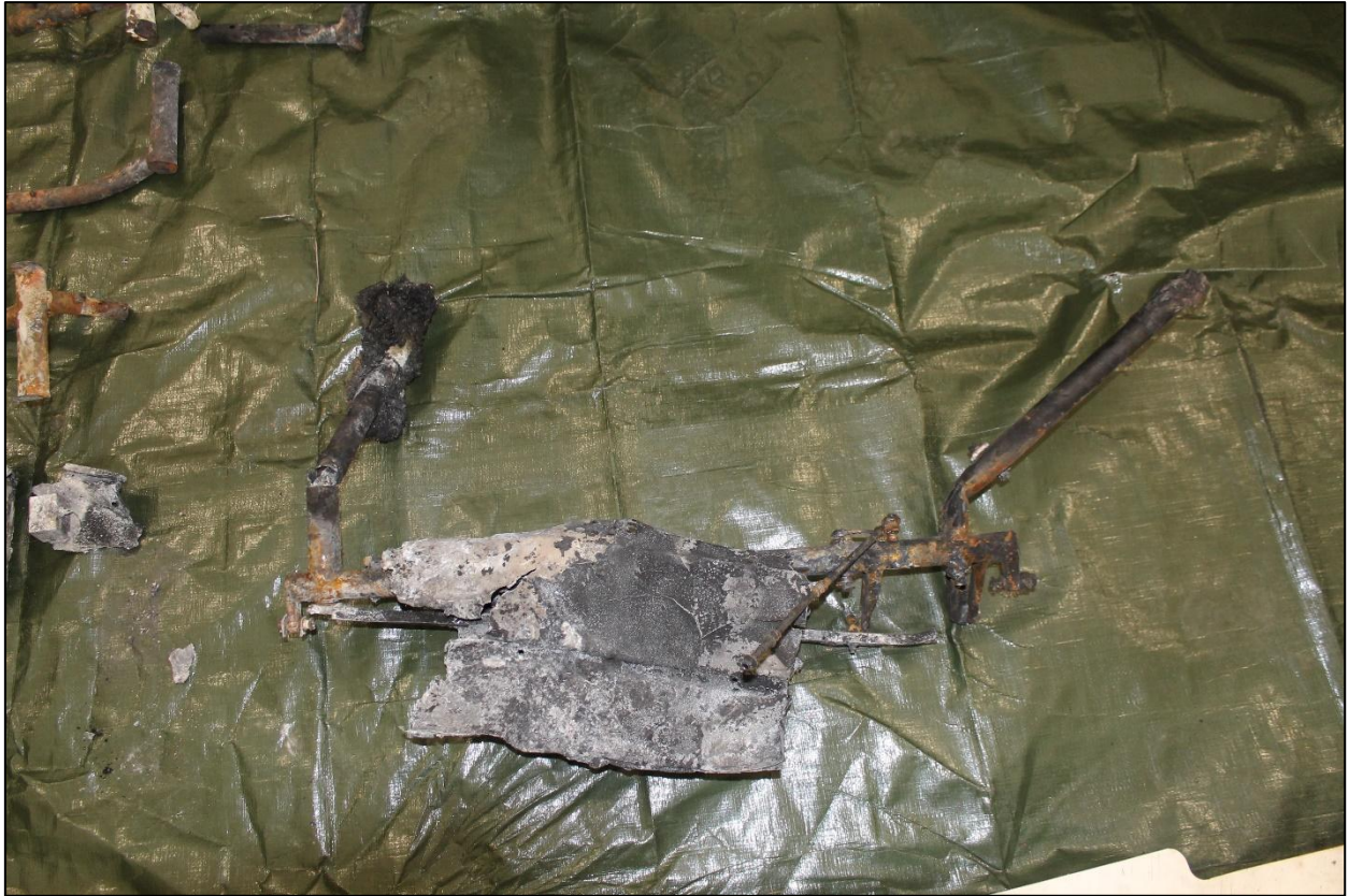
Figure 7. ES-ETR collective lever. (Photo: SIAF)
