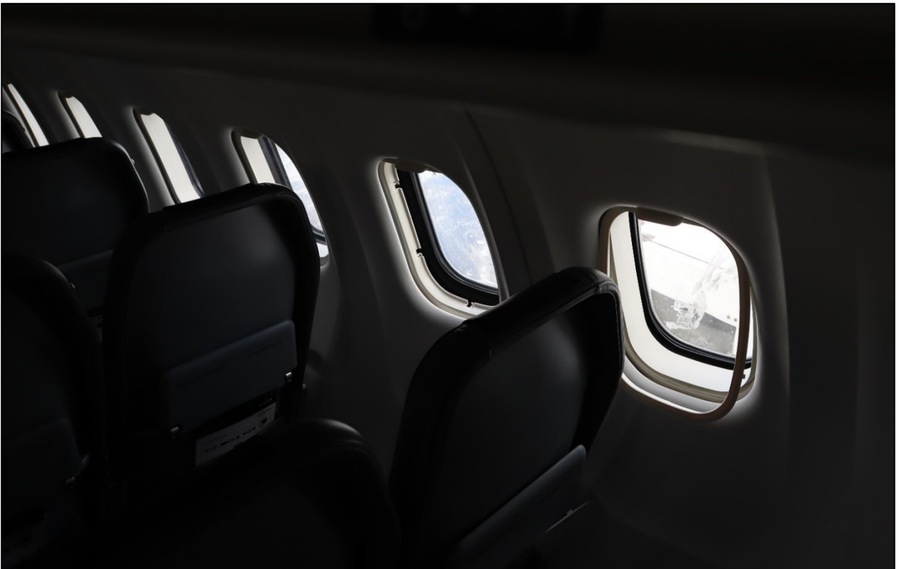
Figure 5. Propeller and GPU fragments struck cabin windows in line with the propeller, dislodging the inner panes complete with frames. (Photo: SIAF)
