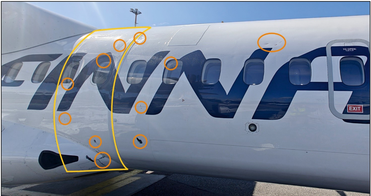
Figure 6. The orange circles indicate airframe damage. The yellow rectangle shows the reinforced fuselage section. (Photo: SIAF)
