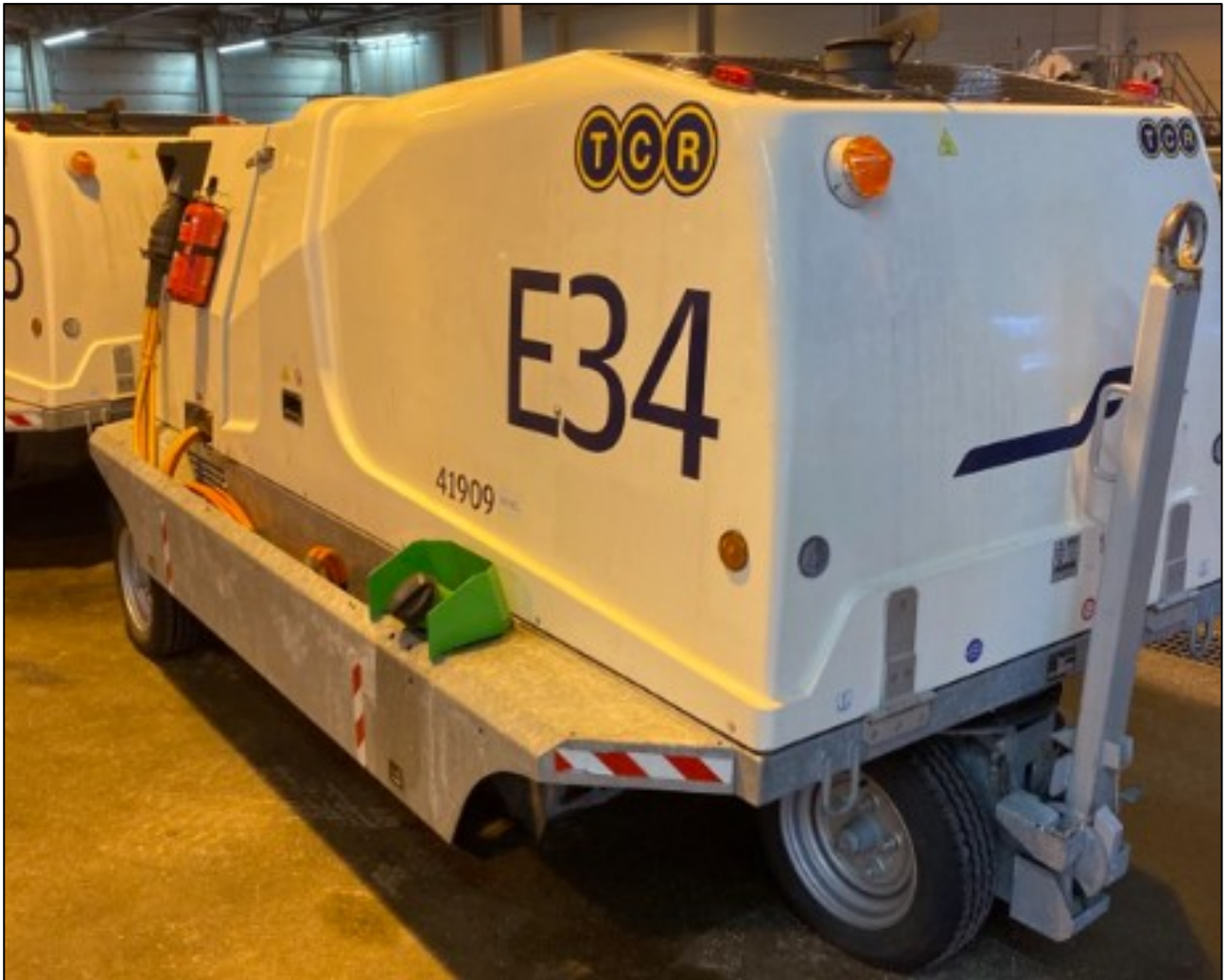
Figure 9. Guinault GA90 ground power unit. (Photo: TCR Finland)
