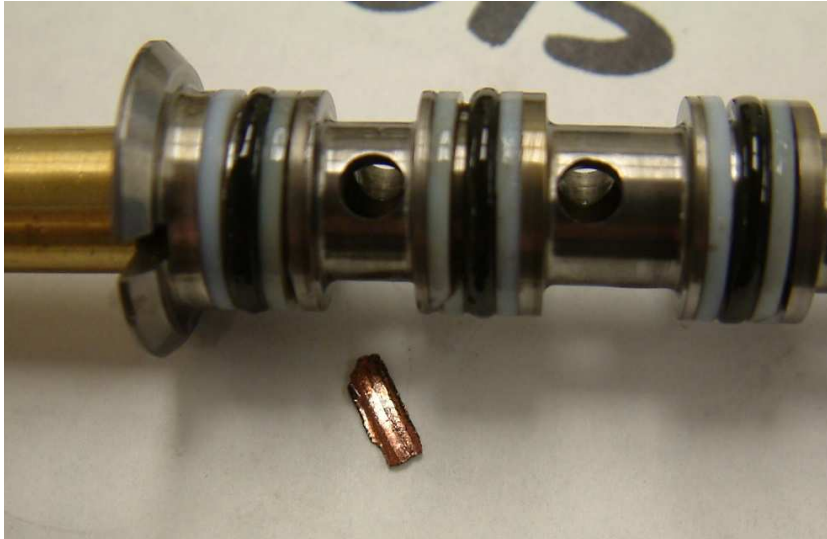
Photo 12. Plasma piece found loose in system no. 2 bypass valve
