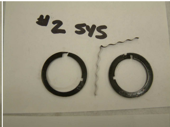
Photo 11. Worn system no. 2 piston head seals.
