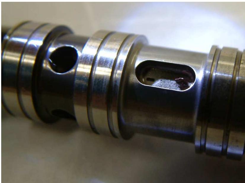
Photo 13. Plasma coating piece(s) in one of the two C 3 return slots of the secondary spool (inner sleeve. The second, not blocked C 3 return slot, is located on the opposite side of the spool and not visible on the photo.)
