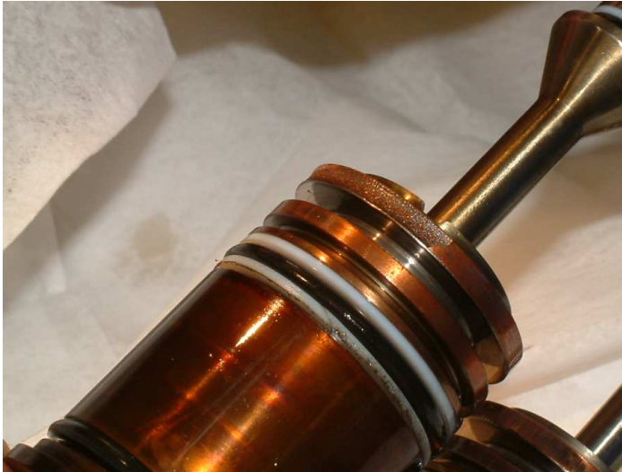
Photo 14. S/N 407 system no. 1 piston with flaked plasma. (Note! This piston is not from accident helicopter.)
