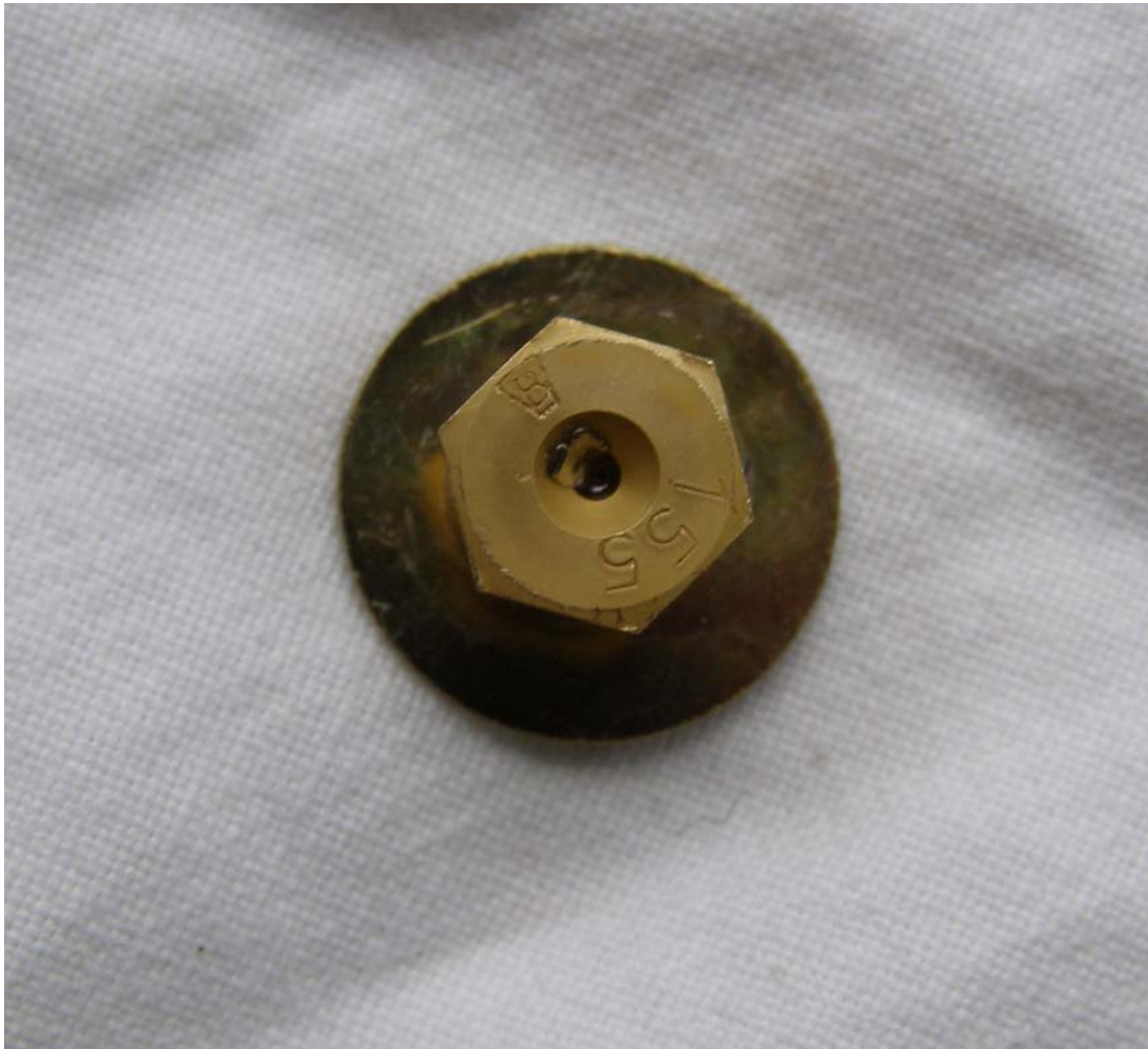
Figure 2.. Metal flakes in the main jet nozzle
