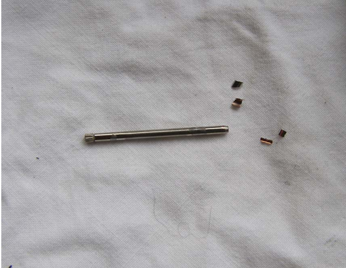
Figure 3. The carburettor pin exhibiting some flaking on its nickel surface coating
