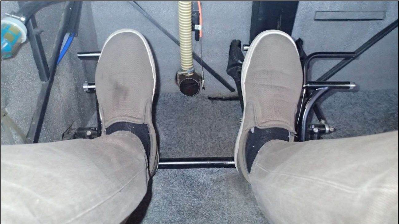
Kuva 2. Correctly positioned feet on a pedal assembly. Photo: SIAF
