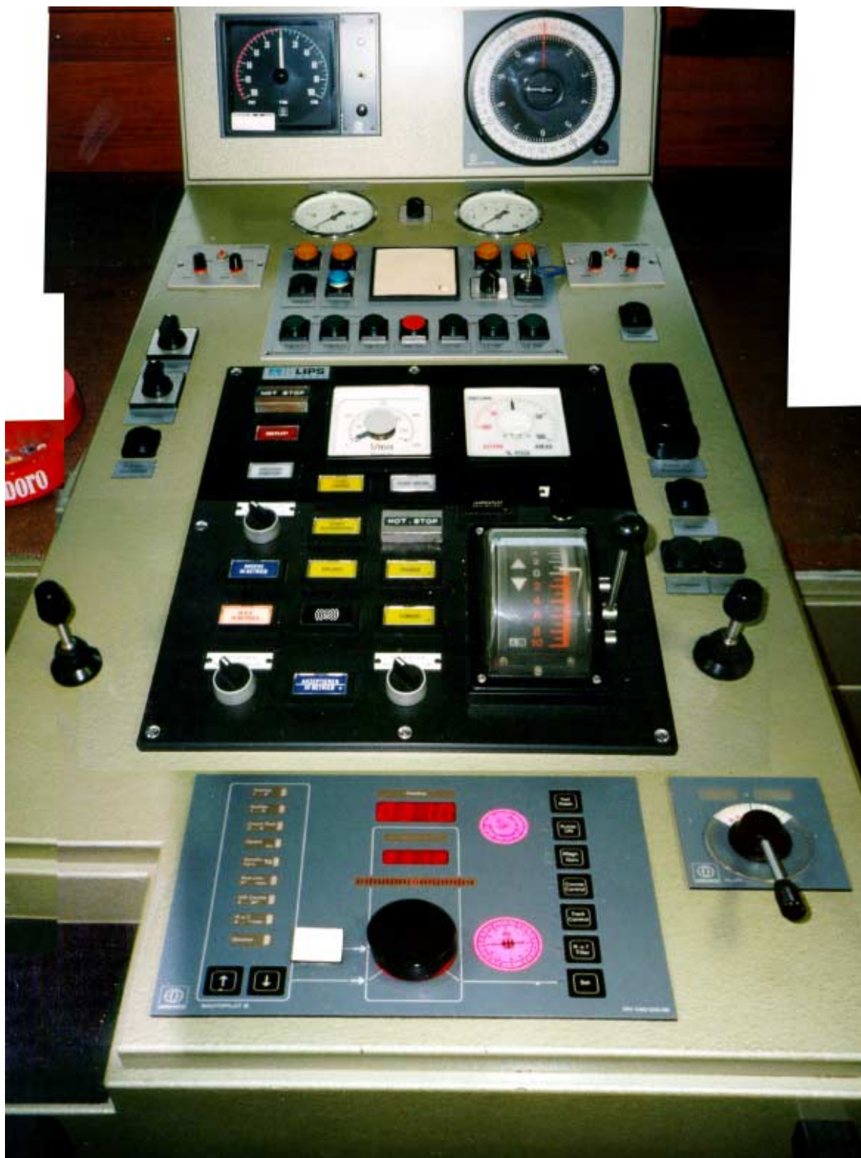
Figure 5c. Middle console of bridge of ms GRIMM. NFU lever used by the pilot is on the left edge.
