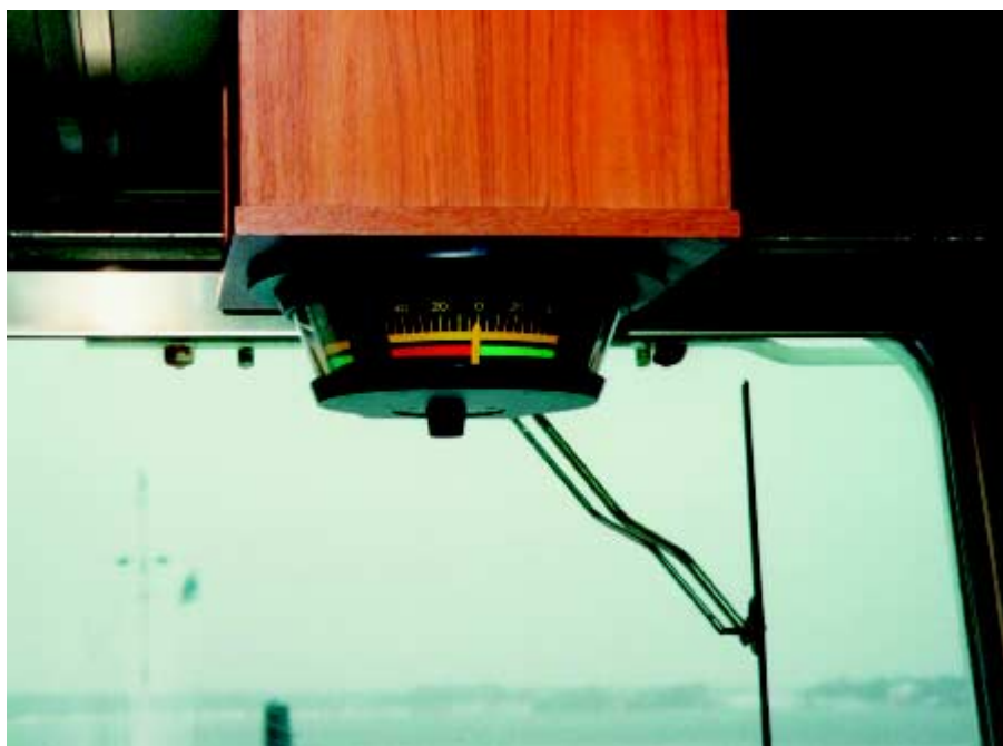
Figure 8b. Rudder angle indicator in ceiling of bridge (Location also seen in Figure 2).
