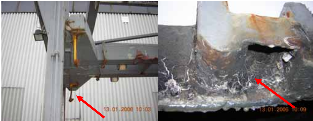
Figure 3. Figure showing the lifting hooks. They deformed as they slid along the pockets and losing the hatch cover. This resulted in toppling over of the hatch crane, injuring the driver of the crane (in three cases resulting in the death of the driver).
