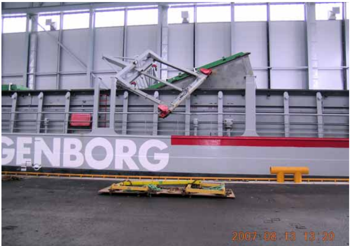
Figure 2. MS GRACHTBORG's collapsed hatch crane.
