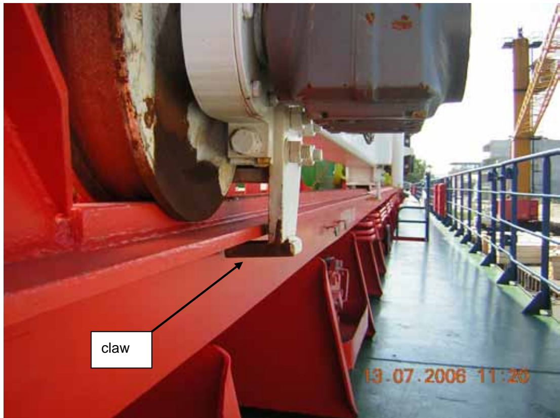
Figure 4. The rail claw, which prevents the crane from derailing or toppling over.
