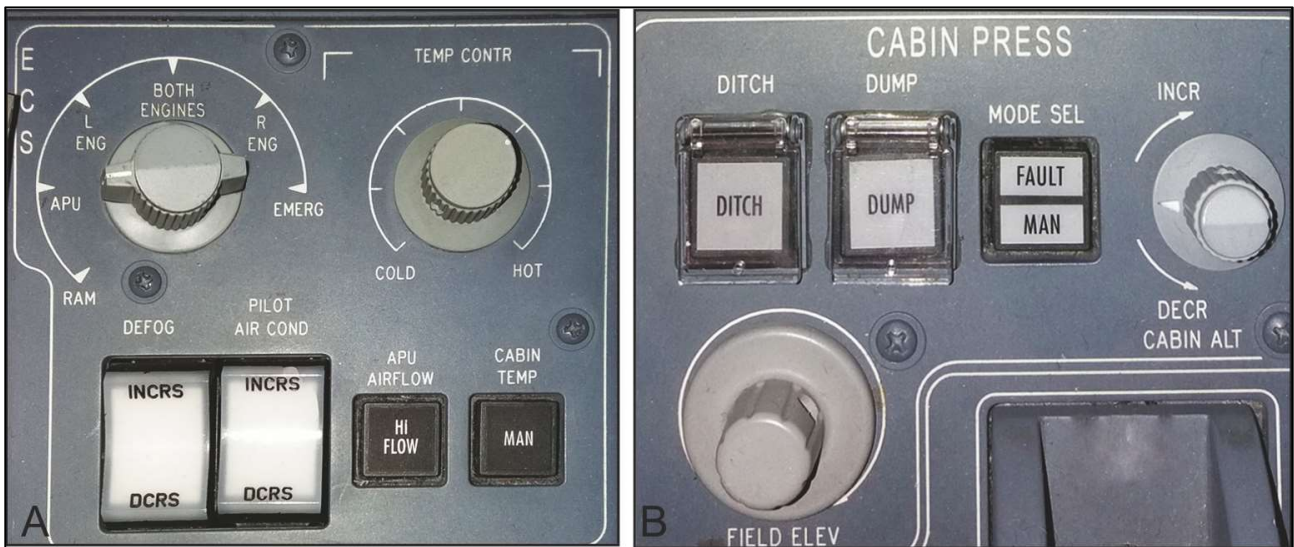
Image 4. 4A: The ECS control panel where the bleed air is selected to APU and the temperature control knob is turned to approximately the one o'clock position. 4B: The Cabin pressurisation control panel. (Photos: SIAF)
